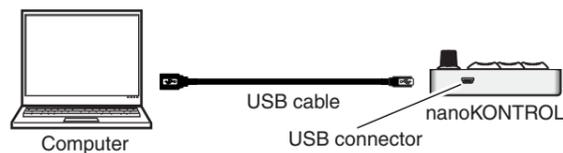
▲ If you're using a passive (non-powered) USB hub, the nanoKONTROL may fail to power-on because it is not getting enough power. If this is so, please connect the nanoKONTROL to a powered USB hub or directly to your computer.
